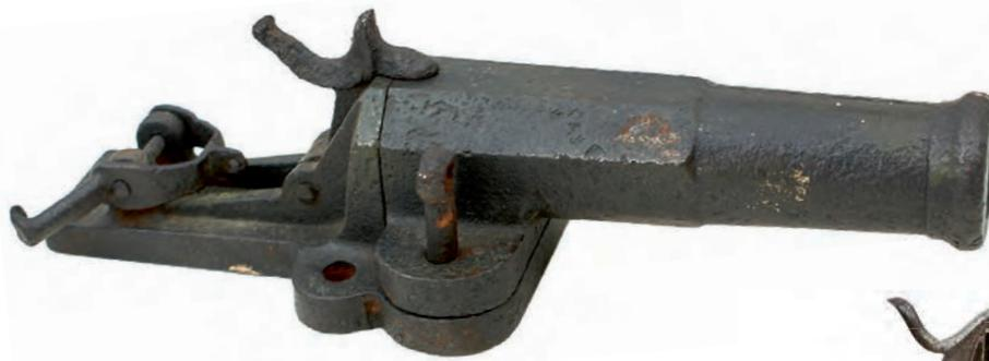
**528.** A LARGE BORE PINFIRE ALARM OR POACHER'S TRAP GUN, 4.75inch two-stage cannon barrel with ring turned muzzle, the cast iron frame with wire guide and two mounting points. £80-100
