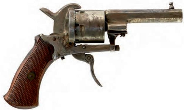
**544.** A 7MM CALIBRE SIX-SHOT BELGIAN PINFIRE REVOLVER, 2.75inch sighted octagonal barrel, loading gate on the right side, the left side of the frame with maker's stamp of Francois Ledant, folding trigger, chequered two-piece wooden grips. Ejector rod lacking. See page 48 of *The Pinfire Revolver Pistol and Ammunition Handbook* by S. Jordan. £60-90
