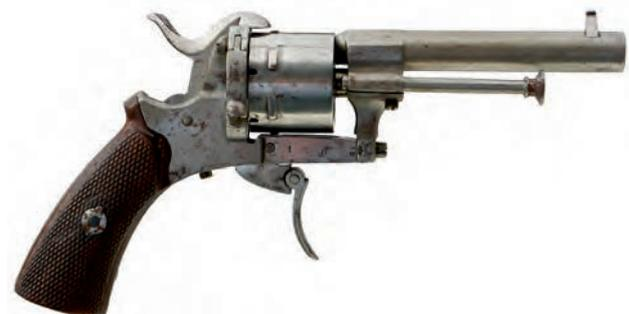
**539.** A 7MM CALIBRE SIX-SHOT BELGIAN PINFIRE REVOLVER, 3.5inch sighted barrel, the cylinder with Belgian proofs, loading gate on the right side, the right side of the frame stamped with the serial no. 150 and a crown over AD, folding trigger, two-piece chequered wooden grips, ejector rod. See page 64 of *The Pinfire Revolver Pistol and Ammunition Handbook* by S. Jordan. £70-90
