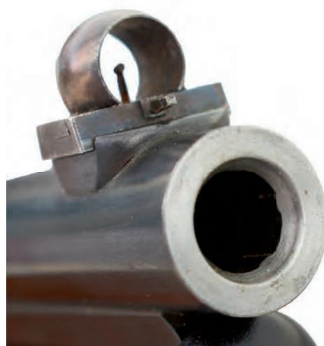
**220.** A GOOD CASED .451 CALIBRE PERCUSSION MATCH OR TARGET RIFLE BY THOMAS TURNER OF BIRMINGHAM, 33.25inch sighted blued barrel, fitted with ramp and ladder rear sights, adjustable fore-sight with key, engraved TURNER'S PATENT, border and scroll engraved case colour hardened breech, border and scroll engraved case colour hardened lock signed THOMAS TURNER & FISHER ST. BIRMINGHAM, half stocked
